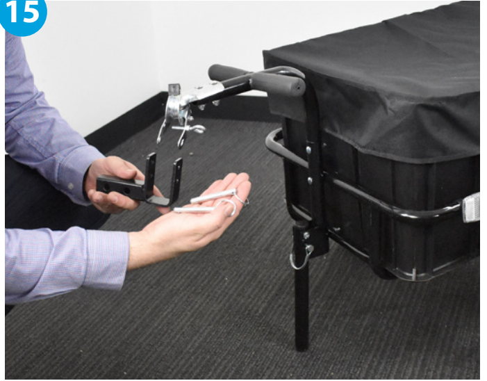
Using two metal pins attach hook and receiver attachment to the trailer hitch as shown in photo
