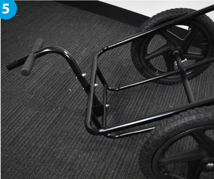
Tighten firmly securing the pole at two points to the trailer frame
